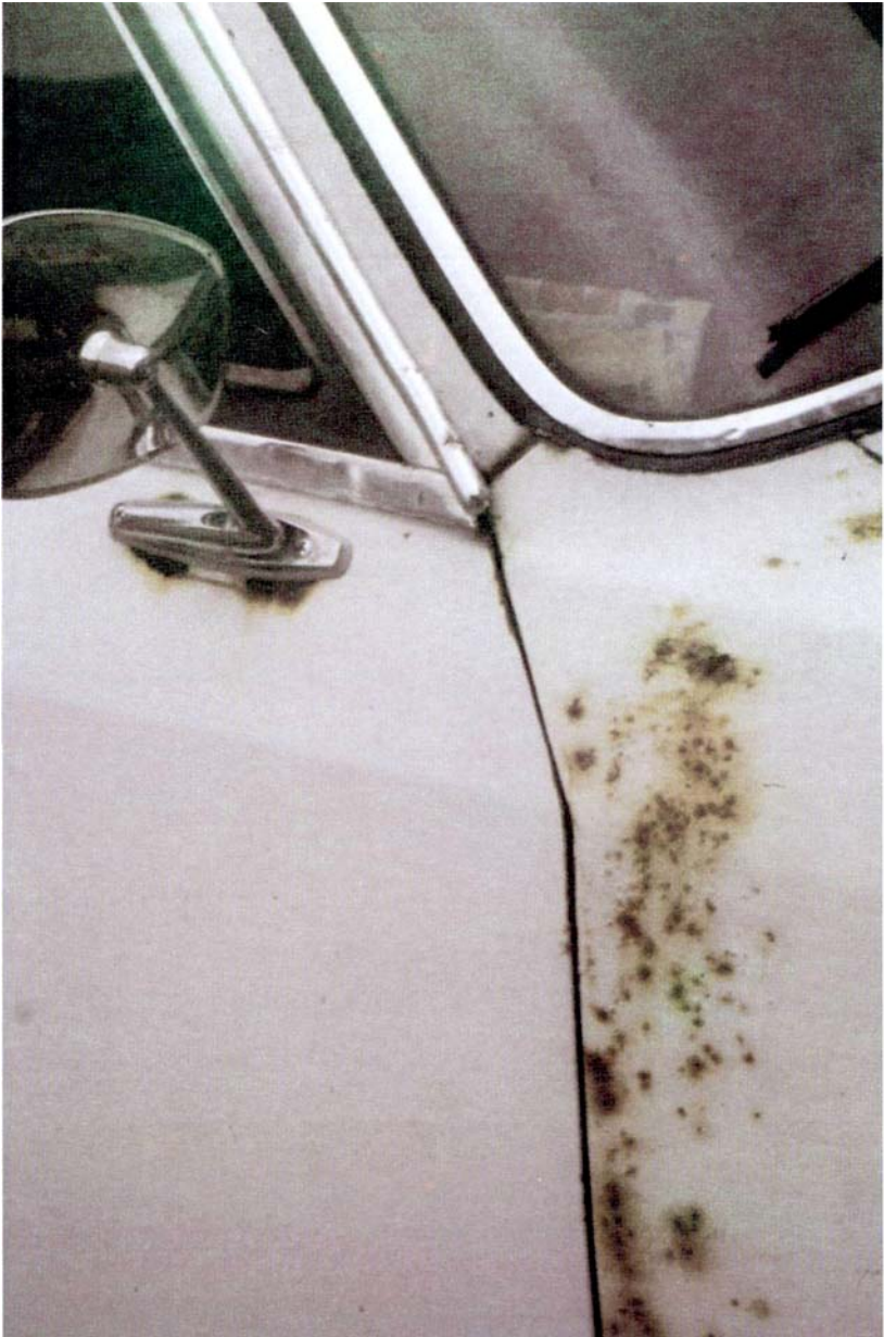
Fig. 28: Deposit corrosion in the front wing of a motor car due to road mud accumulation.
