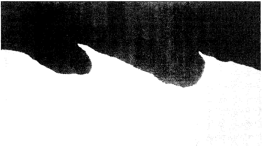
Fig. 34: Cross-section showing attack by erosion corrosion in a copper water pipe; direction of flow from left to right (Metallverken) (x100).
