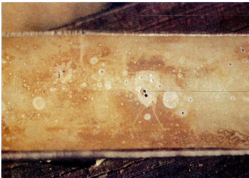
Fig. 120: Pits in a stainless steel pipe (18Cr, 9Ni).
