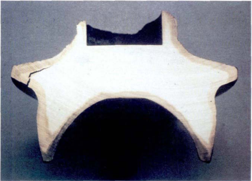
Fig. 30: Cross-section showing dezincification (reddish zone) of a brass valve cone; the attack has arisen during exposure to sea water (Metallverken).
