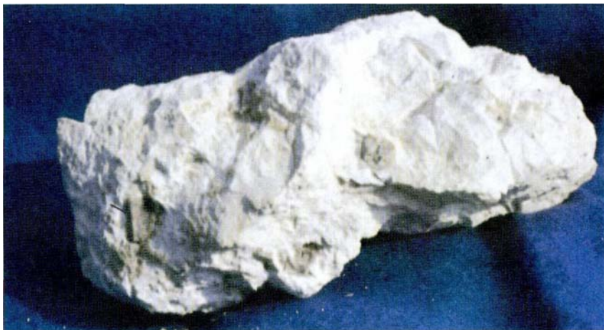
Fig. 14: Fragment from aeroplane wheel manufactured from magnesium alloy which has been completely transformed to a crystalline magnesium mineral after 28 years in the Baltic Sea.
