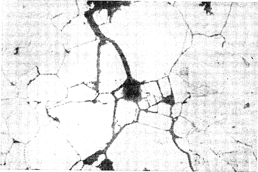
Fig. 38(b): Cross-section showing intergranular cracking (Metallverken) ( \times 500 ).
